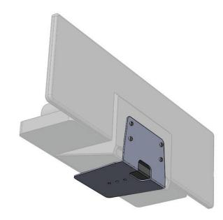
The camera bracket model **BKT-ST60** allows you to mount the Cisco SpeakerTrack60 onto AVFI mounts, tripod or flat surface.
